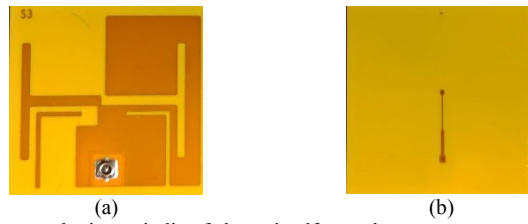
Fig. 13 The prototype of the proposed microstrip line fed quasi-self-complementary antenna, (a) front side and (b) back side.
